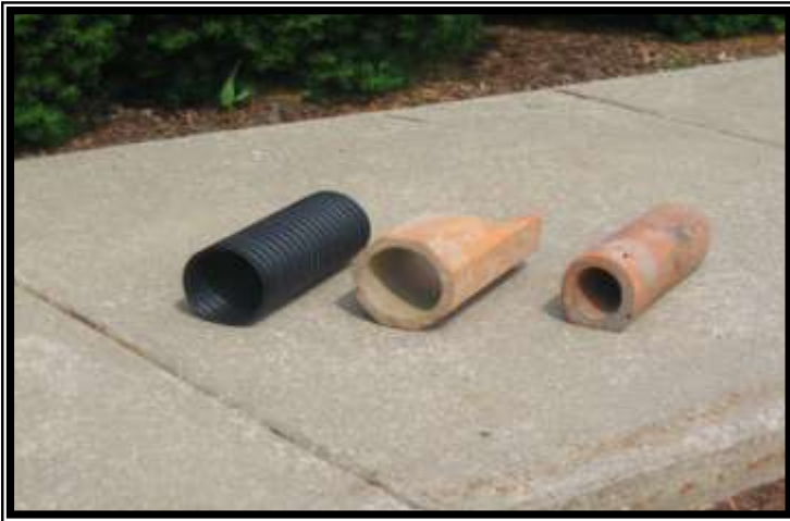
Types of tile. Left to right: Plastic, clay and an old flat bottom clay tile.
